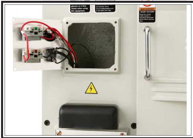
Figure 48. Control Panel & Welder's Lamp.
